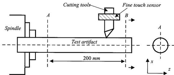
Fig. 4. Diagram of the geometric error measurement of the workpiece using FTS\_Q.
