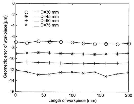
Fig. 5. Geometric errors of the workpiece along the  $z$ -axis.
