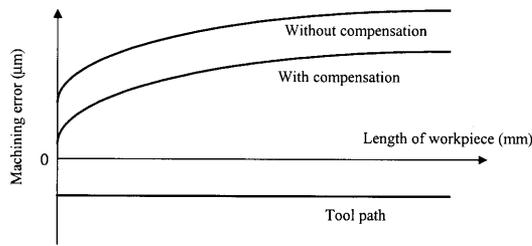
Fig. 7. Compensation of geometric error.
