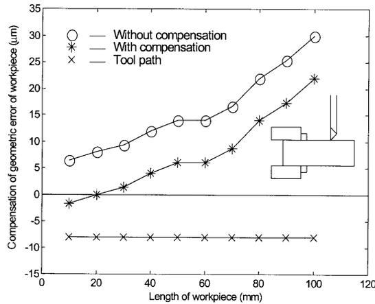
Fig. 8. Compensation of geometric error by a modified NC command.
