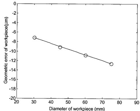
Fig. 6. The average geometric error for the different diameters.
