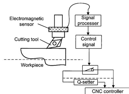
Fig. 1. Flow diagram of a fine touch sensor fixed on a CNC controller.
